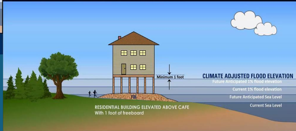
Inundation Risk Zone and Future Flood Elevation
